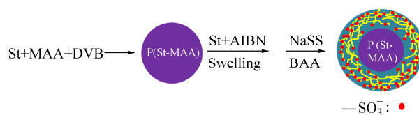
Fig. 1 Synthetic scheme of the x-P(St-MAA)/x-(St-NaSS) core/shell latex particles with high sulphonate contents via seeded emulsion copolymerization
